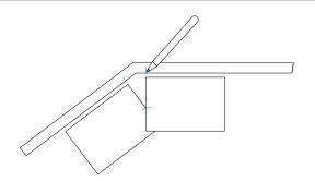
Using a pencil, make a mark on the window sill at the point where the paper meets the window frame.
