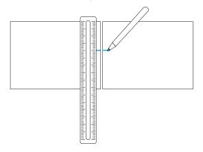
Slide the two pieces of paper towards each other along the window sill of the bay until the two marks that you made meet up.
