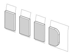
Start by taking one of the pads and, using a pair of scissors, cutting into roughly 10mm segments.
