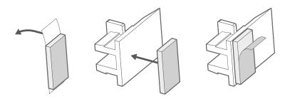
Remove the blind and brackets from the window. Take one of your cut segments, peel off the backing paper and stick the segment to the flat face of the bracket that sits against the glass. Peel off the protective film on the front of the segment, then carefully reinsert the bracket in the window. Press each bracket firmly against the glass for around 30 seconds once reinserted, to allow the adhesive on the grip pad to bond.
