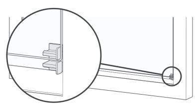
Slot the brackets back into the corners, as per step 1 of this quide.
