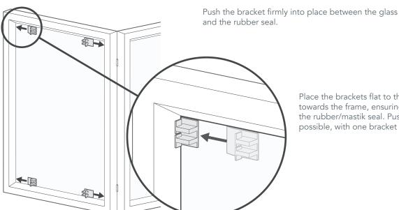
Place the brackets flat to the glass and push them in towards the frame, ensuring that they slide in under the rubber/mastik seal. Push in each bracket as far as possible, with one bracket in each corner of the glass.
