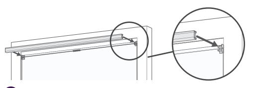
Click the two separate rails onto the brackets at the top and bottom of the window. Simply line up each rail's open side with the brackets and push firmly until it clicks into place.
