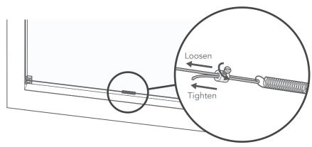
At the bottom of the blind the cord is connected to both ends of a small spring. On one side, the cord is secured by a metal sleeve with a screw.
