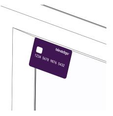
To correctly locate the brackets, take a standard sized debit or credit card and hold it in the corner of the glass.
