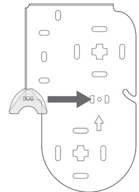
On the side where the controls will be, clip the chain runner attachment into its slot near the middle of the bracket.
