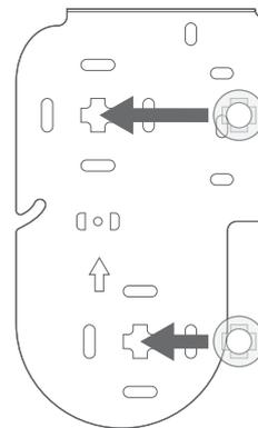
On the bracket opposite to where you'd like the controls, clip the circular attachments into the two cross cutouts in the bracket.
