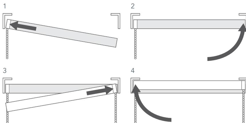
Install the rear blind first. Begin by placing the spring-loaded pin into the lower circular hole on the bracket. Push the blind toward the bracket so the spring-loaded pin depresses.
