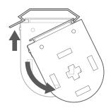
To release the blind from the brackets at any point after installing, push up firmly against the tab protruding from the back of the bracket. At the same time, twist the back of the headrail downwards to disengage it at the back.
