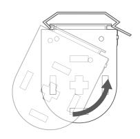
Push the back of the headrail upwards to lock it into the back of the bracket.
