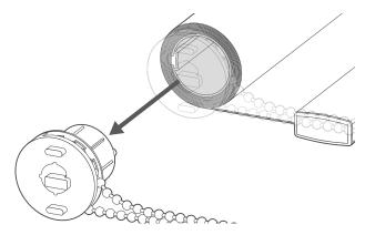
Lay the blind down and gently pull the sidewinder mechanism out of the roller tube. You won't need this mechanism after you've installed the motor, but we'd recommend keeping it safe somewhere for future use, just in case.
