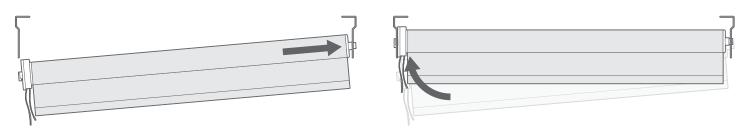
Locate the depression end (the opposite end to the controls) of the blind into the circular hole in the corresponding bracket. Lift the control end of the blind and slot the locking pegs into the corresponding slots on the bracket.
