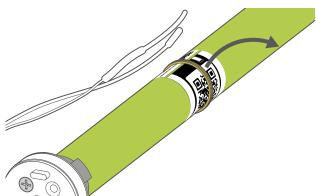
Unpack the roller motor - you'll find a label containing a QR code secured to the motor with an elastic band. Remove the label and set it aside for later.
