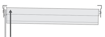
Then, push the blind toward the opposite end to release the control end from its bracket entirely.
