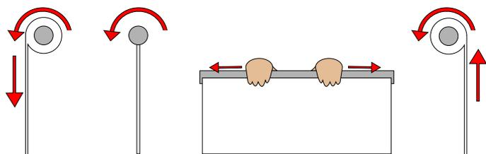
If you wish to change the roll method, unroll the fabric fully so that you can see the aluminium tube. Keep turning the tube in the same direction so that the fabric starts to roll up on the opposite side. Run your hands along the fabric to loosely form a fold so that the fabric sits closer to the tube and continue rolling the fabric back up.
