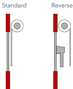
Roller blinds can have the fabric rolled onto the tube in two directions. The first is referred to as a 'standard' roll. This will place the fabric closest to the window or wall so that it comes down at the back of the tube. This is typically used with blackout blinds when they are mounted outside of a recess, the standard roll meaning that there is less light leakage.
