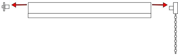
We will have positioned the controls where you requested during the ordering process. However if you decide to swap the side that they are on, direction of the roll or need to trim the blind further, the controls can be removed by simply unplugging them from the tube. This should be done prior to fixing the brackets.
