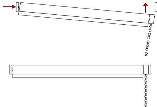
When the brackets have been fitted to the window area, locate the 'pin' (the end of the blind opposite to the controls) into the bracket first. Then fix the control end into the opposite bracket.
