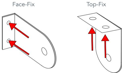
The brackets that are supplied with your blind enable you to face-fix the blind onto a wall/window frame, or top-fix the blind onto the ceiling/underside of a recess.
