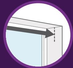
Top-fixing or face-fixing are recommended for most installations, whereas **side-fixing is only recommended if the width you gave us was taken right at the top of the recess.**
