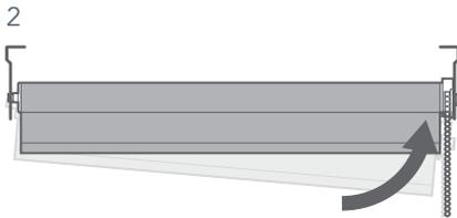
Keeping the pin depressed, lift the sidewinder end of the blind upwards so the blind is level and the chain is hanging directly down from the bottom of the sidewinder and slot the pegs of the control into the cross section of the bracket.
