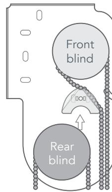
Take the chain for the top (front) blind and drape the back part of the chain over the chain runner so that the chain sits forward, preventing it from tangling with the other blind's chain.
