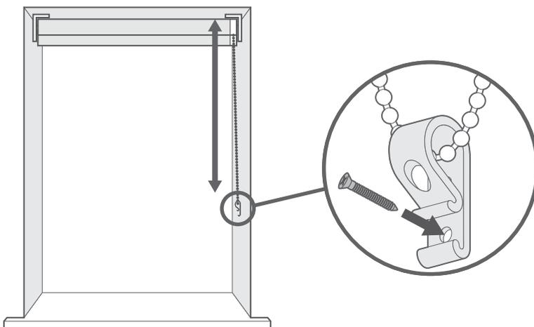
The cord retaining device must be installed at the maximum distance possible from the control mechanism to prevent looped cords from becoming slack.
