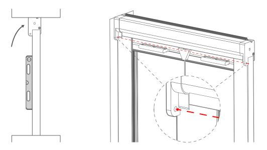
Place the screen in position in the recess, using a spirit level to make sure it's straight. At either end of the blind's cassette, you'll see a fixing hole - mark through the hole onto the wall on both sides with a pencil.
