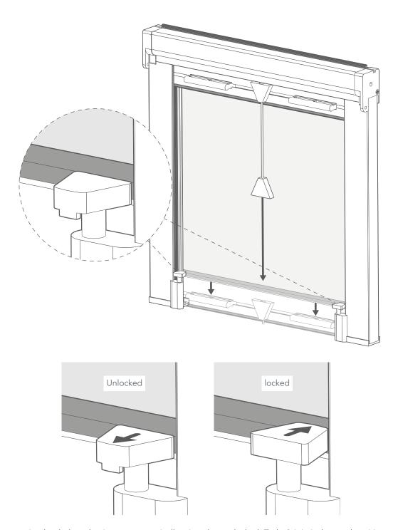
The blind uses a spring-loaded mechanism to automatically raise when unlocked. To lock it in its lowered position, pull the cord to bring it down, then hold it down at the bottom with the two tab handles and use the locking hooks on the bottoms of the side channels to fasten it in place.
