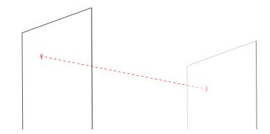
Take the blind back down and drill a hole into the wall at each side of the recess. Insert a wall plug into each hole.
