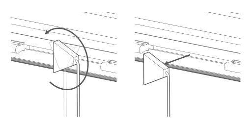
If you'd prefer not to have the pull cord on the front of the blind, this can be easily removed. Simply twist the cord mount on the front of the bottom bar in either direction then pull it out of the bar. Now the bar can simply be raised and lowered using the two handles.
