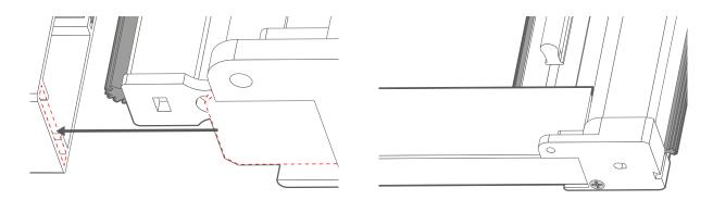
Lay the blind face up and slot the side frames onto the ends of the cassette - there is a slot at the top of the frame you can use to line it up correctly with the end of the cassette.
