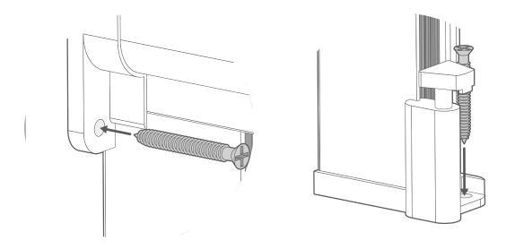
Lift the blind back into position. Use one screw at each side to secure the casette in place. Secure the side channels directly to the sill using one screw for each channel.
