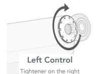
Hold the blind securely in place and turn the tightening wheel to tighten the blind in place.
