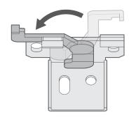
Hook the front lip of the headrail over the protruding hooks at the front of the bracket, then raise the back of the headrail so that it's level. Holding it in this position, swing the swing-arm over and press it firmly against the headrail to lock it in place.
