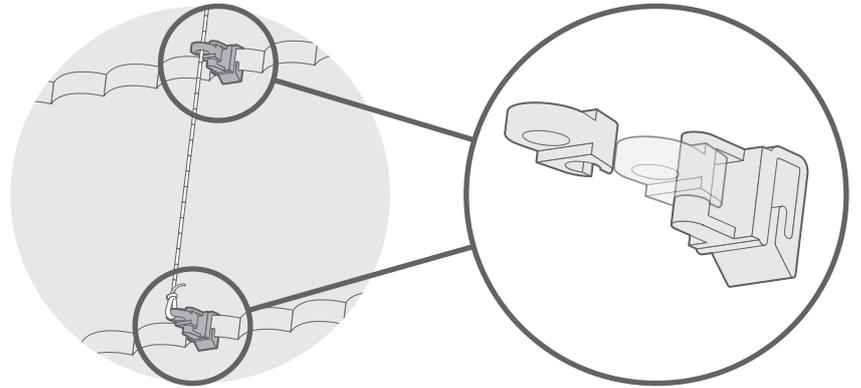
At the back, the cords attach to the fabric using clips, which double as a child-safety feature. These clips are in two parts, and can be easily unclipped to separate the cords from the fabric.
