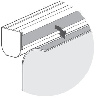
The fabric attaches at the front with velcro, simply peel the fabric away from the headrail.
