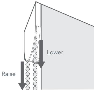
Pull down on the front part of the chain to lower the blind, and pull down on the rear part of the chain to raise the blind.
