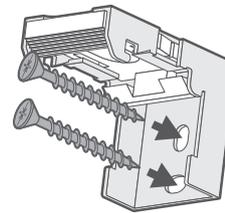
Where the brackets are screwed onto a facing surface (a wall or window frame)
