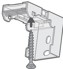
Where the brackets are screwed into the lintel (or 'ceiling' of the recess)
