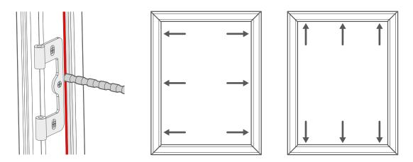
Pre-drill fixing holes through all four frames. The holes should be drilled through the channels along the inside face of the frames. On the sides, shere should be one hole level with each hinge and one in the centre. For the top and bottom, drill them a similar distance in from each end, and one in the middle again.
