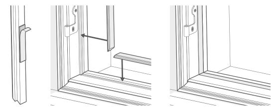
Start with the inner frame trim. Peel the covers off the sticky pads on the back of the trim pieces. Slot the trims into the channels through which you inserted your screws. This will cover the screws.
