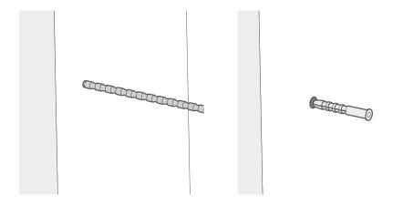
Remove the panels and frame from the window, then drill holes where you made your marks. Insert a Rawl plug into each hole.
