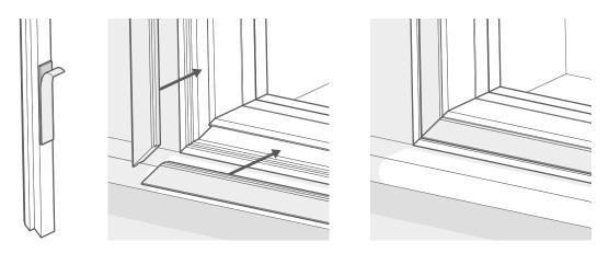
Peel the covers off the sticky pads on the back of the trim pieces. Slot the outer trim into the channels on the front face of the frames.
