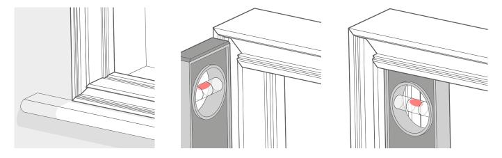
Slot the assembled frame into the window, using a spirit-level to make sure the frame is level. Check all four corners to ensure the frame isn't tipped or twisted at all.
