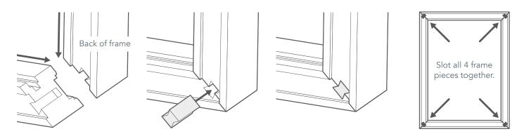
Start by slotting the frame pieces together, then secure them using the provided Hoffman keys.
