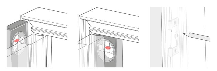
With the panels in place, take a moment to re-check that the frame is level in all corners. Pack the blind tighter into place if necessary, once level. Mark through the screw holes in the frame, onto the wall, with a pencil.
