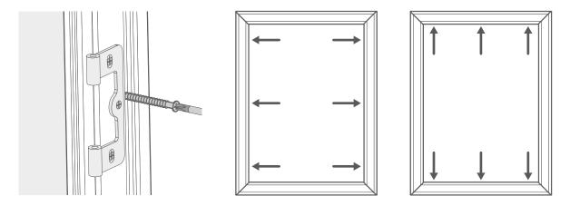
Place the frame back into position in the window and screw into place using the long screws provided.
