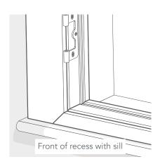
For front of recess (and front of recess with sill) fitting, a wider trim is supplied that is designed to overlap onto the wall around the recess.
