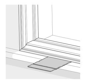
Once you're happy that the frame is level, pack the frame out to prevent any movement. The easiest way to do this is to use pieces of the box your Shutter arrived in, layered between the frame and the walls and sill.
