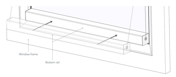
Pull the bottom rail out towards the bottom of the window, stretching out the cords. Just like the top rail, line up the bottom rail carefully with the edge of the visible glass and press it into place.
