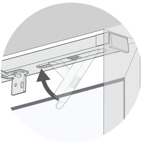
Hold the Click2Go™ rail up against the top of the recess, then push the lever firmly upwards until the rail snaps into place. If the rail is not quite tight enough then this can be easily adjusted:
