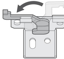
Hook the front lip of the headrail over the protruding hooks at the front of the bracket, then raise the back of the headrail so that it's level. Holding it in this position, swing the swing-arm over and press it firmly against the headrail to lock it in place.
