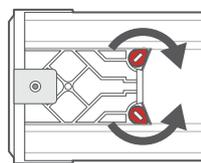
At the end of the rail opposite to the lever there is an adjustment block that allows you to fine-tune the fitting of the rail. Use a flat-head screwdriver to twist the small red plugs **in** toward the centre of the rail. Slide the block out of the rail by a few millimetres, then twist the red plugs back into their original position to fix the block in place. **Make small adjustments only**, repeating as necessary for a tight fit.
