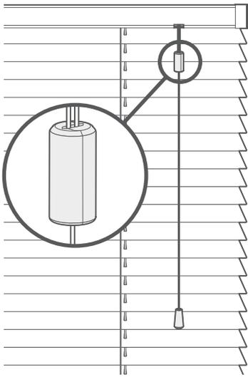
A breakaway cord condenser is pre-fitted to the lift cords so that when a horizontal force is applied to the cords above the condenser, it safely breaks away, eliminating any hazardous loops.
