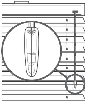
A breakaway cord condenser is pre-fitted to the lift cords so that when a horizontal force is applied to the cords entering the condenser, it safely releases the cords to eliminate any hazardous loops.
