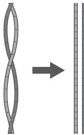
... Then simply click the two halves of the consolidator back together, ensuring there are no loose threads caught between the edges.
