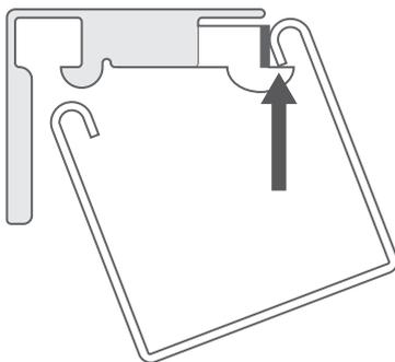
Situate the front lip of the headrail into the front of the bracket.
