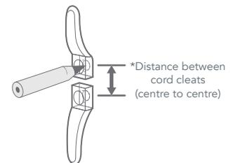
Mark the hole positions and drill as required. Use the screws provided to attach the safety cleat to the wall.
