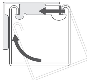
Push the back of the headrail upwards to lock it into the back of the bracket.
