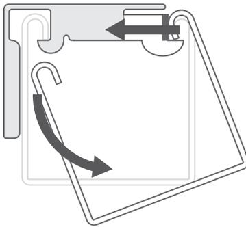
To release the blind from the brackets at any point after installing, push firmly against the blind's headrail to disengage it from the back of the bracket. At the same time, twist the back of the headrail downwards to release it.
