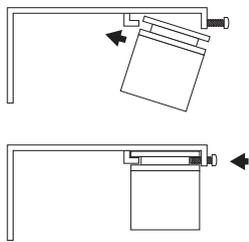
Rest the rear ridge of the rail into the hook on the bracket. Lift the front of the rail up so that it sits flush with the bracket and tighten the front screw so that it secures into the front ridge of the rail.
