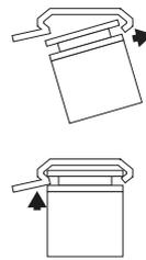
Rest the front ridge of the rail onto the front lip of the bracket. Lift the back of the rail to meet the bracket and press firmly upwards so that it clicks into place securely.
