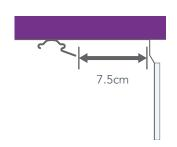
If you're using top-fix brackets, make sure that you mount them at least 7.5cm in front of either the window frame, or any protruding vents or handles, if there are any. This allows space for the louvres to turn open and closed.
