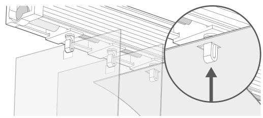
To hook the louvres onto the rail, simply hold upeach louvre and feed the square hole in the top over the hooks in the rail, then allow the louvre to straighten and hang.
