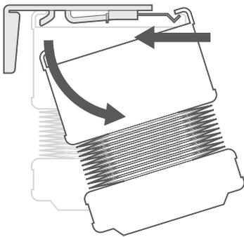
To release the blind from the brackets at any point after installing, push firmly against the blind's headrail to disengage it from the front of the bracket. At the same time, twist the back of the headrail downwards to release it from the back.
