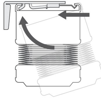
Push the back of the headrail upwards to lock it into the back of the bracket.
