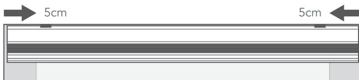
The outermost brackets should be mounted at least 5cm in from the ends of the blind. Any remaining brackets can be spaced evenly across the width of the blind.
