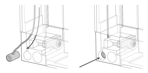
On both sides, feed the cord down and out the bottom of the side channel. Then, insert the barrel on the end of the cord into the outermost hole in the bottom corner piece. Insert the barrel so that the inset tightening screw is facing you.
