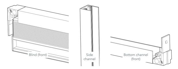
The side channels will slot onto the pegs of the corner pieces. The corner pieces are already slotted into the ends of the blind and the bottom channel for you.
