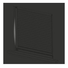
Most recesses are not perfectly straight and level, so before going any further, pull the blind's handle down until the blind is fully lowered. If you notice any light leakage around the light seals, there should be enough excess seal left over for you to remedy this by attaching a matching strip to the inside of the recess at the back of the blind.
