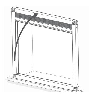
Lift the assembled blind into place over the recess, making sure it's straight and level.
