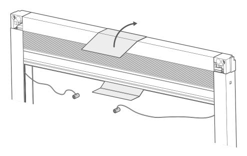
Remove the wrapping from the blind to release the cords. The wrapping can be disposed of.
