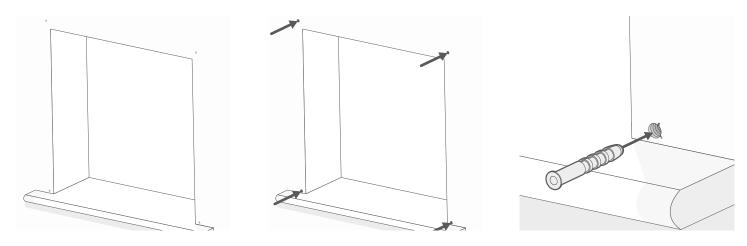
Drill a hole at each of your marks, then insert a Rawl plug into each hole.
