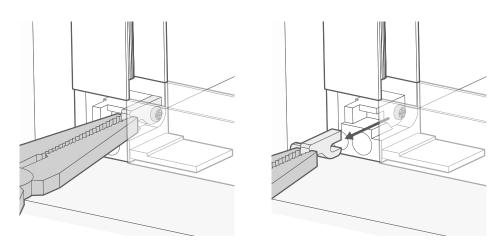
Once you're happy with the blind's position, use a small pair of pliers to pull the spring stopper from each corner piece. The spring-loaded mechanism in the corner piece will engage once the stopper is removed, securing the blind to the walls of the recess. Remove the stopper from all four corner pieces. **Keep the stoppers somewhere safe in case you need to remove the blind from the window for any reason in the future.**
