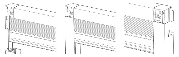
Lay the blind face-up on a clean, flat surface. Slot the side channels onto the blind's corner pieces - they are intentionally a tight fit, so you may have to push quite hard to slot them securely into place (twisting the channels a little as you push also helps). You should hear the corner piece 'click' into place when pushed in hear the corner piece 'click' into place when pushed in far enough.
