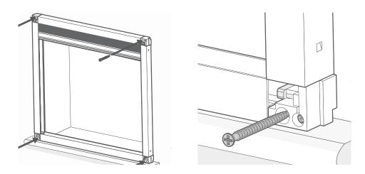
Lift the blind back into position and screw it into place. Take care not to over-tighten the screws.
