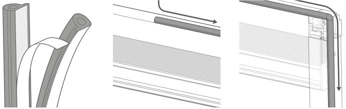
Start by fitting the light sealing strip to the blind. The strip is provided on a long roll with its two halves joined together. Split the two halves, peel the adhesive cover from one end and stick it to the blind's frame. The strip should attach to the outer surface of the blind's frame, with its rounded front aligned with the front edge of the frame.
