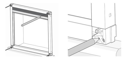
Holding the blind steady, use a pencil to mark the positions of the screw holes. There's one screw hole in each corner piece.
