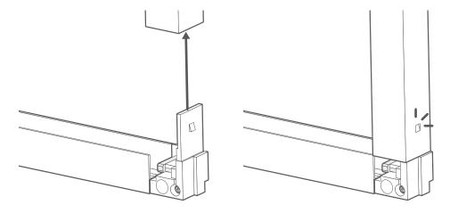
Now slot the bottom channel onto the side channels in the same way.
