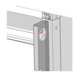
Lift the assembled blind and slot it into place inside the recess, making sure that it's straight and level. Use a spirit level on both sides of the blind to make sure there's no tilt or twist to it.
