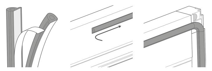
Start by fitting the light sealing strip to the blind. The strip is provided on a long roll with its two halves joined together. Split the two halves, peel the adhesive cover from one end and stick it to the blind's frame. The strip should attach to the back surface of the blind's frame, with its rounded front facing outwards.
